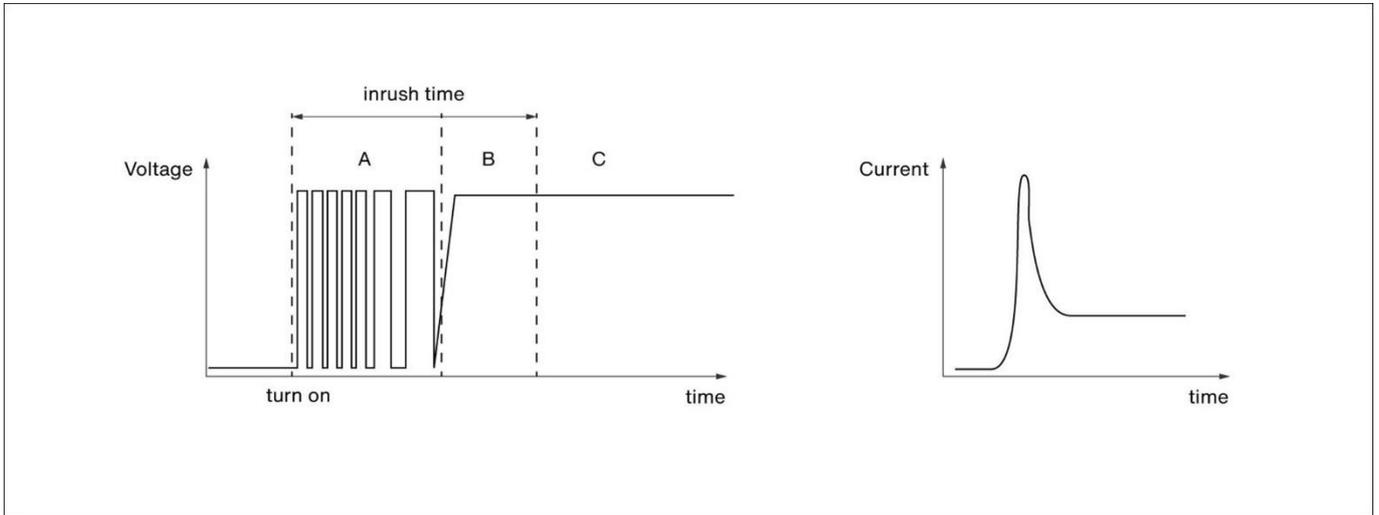
Figure 19: Capacitive soft start
